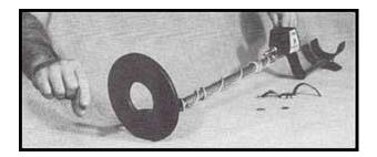
We are now ready to discriminate targets from each other. We will start with the DISCRIMINATE LEVEL at MIN. Please notice that the DISCRIMINATE LEVEL knob has words that correspond to the items that are discriminated out. There is also an arrow between Iron and  $5\phi$ . This is the recommended discriminate level when using the notch filter. This manual will go more into detail about that in the "Set Notch Window Width" section.
