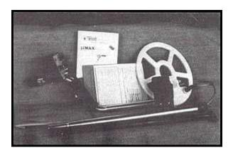
Assembly of the Golden  $\mu$ Max is simple and requires no special tools. Just install the battery, mount the searchcoil on the lower pole assembly, connect the two pole assemblies together, wrap the excess cable around the pole and plug the cable into the control housing. Finally, adjust the pole length and searchcoil angle and you're ready!
