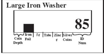
The thing that both of these illustrations have in common is that various segments of the display do not "agree" with each other. This is a sure sign that you are detecting an odd-shaped piece of iron. Notice on the rest of the illustrations that the bar graph and the ID number show about the same information. When the ID number and the graph "agree," you can be sure that your DeLeón is receiving a clean signal.
