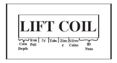
Below are some of the possible readings from various targets. These are not exact and your machine may read slightly different. Take the time to learn the readings and responses for your machine, both in the air test and in the ground.
