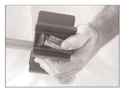
Remove the batteries by pressing down on the right side of the 4-pack battery holder so that the left side of the holder will pop up. Pull out the holder and replace the batteries as needed.
