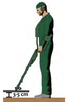
e. In such a case, raise the search coil to a distance of 40 cm again. Press the “ - “ button a few times and leave after reset. Approach the search coil to the ground by the same distances again. If the lights are on and if the sound alert continues (and the number of the lights on will reduce after every action) these actions should be continued until the effect is lost.
