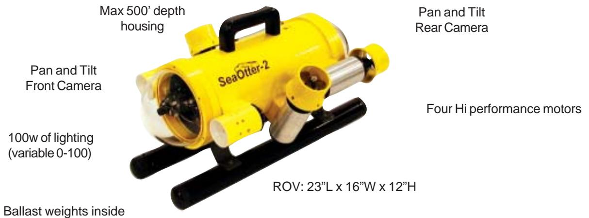
The two skids contain ballast weights that are used to adjust both the balance and buoyancy of the ROV in water. When properly adjusted, the ROV should sit level in the water and should be slightly positive, just positive enough so it does not sink (extra ballast weights are included.)
