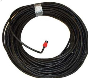
The umbilical cable connects the ROV to the control box. The cable is neutrally buoyant and has a connector on both ends. The system comes standard with a 250 foot cable. Additional cable can be ordered up to a total length of 500 feet (do not exceed this total length.) When additional cable is ordered it comes with a connector on both ends and performs as an extension cord. The additional cable installs between the 250 foot cable and the ROV.
