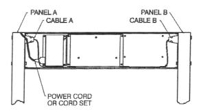
3.2.5 Use the remaining screws and washers to attach the Crosspiece to the two panels, as shown.
