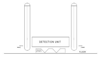
3.2.4 Open door of the Detection Unit and, first, connect Power Cord. Then, connect Cable A and Cable B to the Panels as shown.
