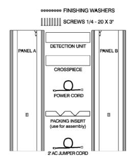
3.2.2 Install the Power Cord completely through one of the channels at the top of either of the Panels as shown below. A channel can be found in each of the four corners. Select the corner that will be convenient in relation to site selection. For overhead power connection, do not insert the cable through a channel but leave it free at the top.
