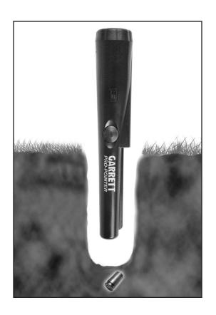
**Side-Scan Recovery:** One of the key features of the Garrett *CSI PRO-POINTER* detector is its side-scan detection ability. This feature allows you to quickly search a large area. Hold the *CSI PRO-POINTER* on its side, flat against the ground and quickly scan back and forth. Once the general location of the target is known, use the tip of the *CSI PRO-POINTER* to precisely locate the target. In addition, you can use the scraping blade to rake, scrape or flatten the soil while side-scanning.
