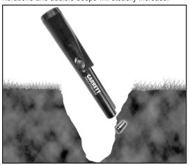
If you do not receive a response from inside the hole or the soil/plug that was removed, the object is likely deeper in the ground or deep inside the plug—beyond pinpointing range. Sweep with your ground search detector again to confirm where the object is.
