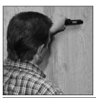
(Left) For wall scanning with a PRO-POINTER, use the sidescan technique to quickly cover large areas.
