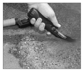
**Wall Searches:** The *CSI PRO-POINTER*'s static mode makes it an excellent utility locator to find objects hidden in tight spaces and to pinpoint projectiles that may have become embedded in a wall. Use the side-scan technique to quickly cover large areas and use the pinpointing tip to precisely locate the target.
