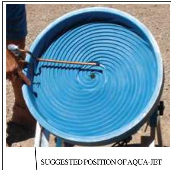
The aqua-jet is positioned simply by bending it to get the stream of water aimed into the clump of side the wheel. NEVER POINT THE STREAM DIRECTLY INTO THE SPIRAL RIFFLES!
