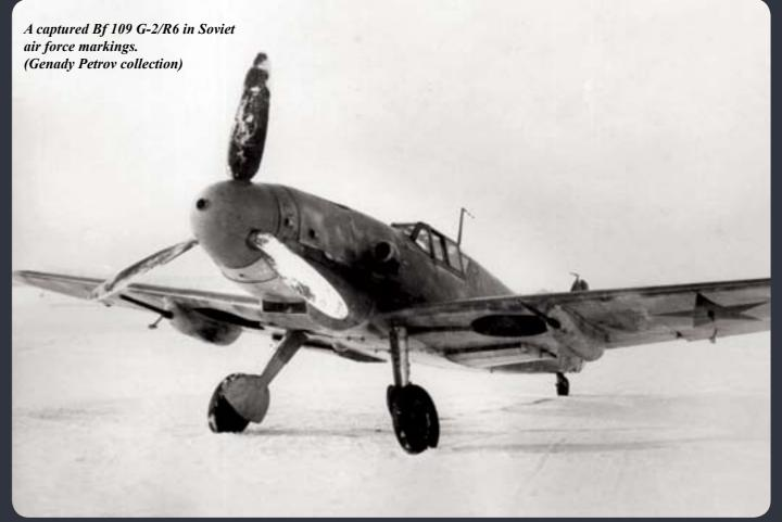
109G-0 machines with Werknr. 14001 to 14003 was delivered over 1942 although still fitted with a DB-601 engine since the DB605 was not yet available. Soon more versions followed, designated as Bf 109G-1 (the first one being Werknr. 14004) to G-16. By early 1943 most Bf 109F's had been replaced by the G-variant.
