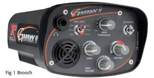
The detector switches on as you start to turn the sensitivity switch clockwise, and as you continue to turn the knob, the sensitivity of the detector increases. There is a red marker at 3 o'clock showing the recommended setting. These red markers are also found next to the other controls, indicating XP's recommended factory settings.
