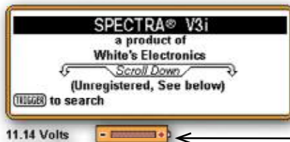
Battery Voltage Reading
