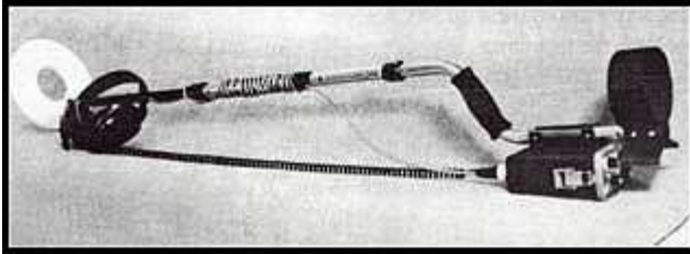
Control housing mounted under arm
