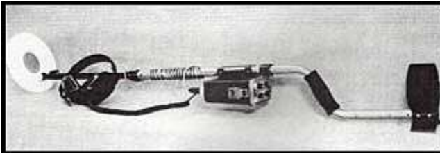
Control housing mounted under pole
