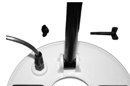
Figure 3 – Pole Tip In Searchcoil Mounting Ears
