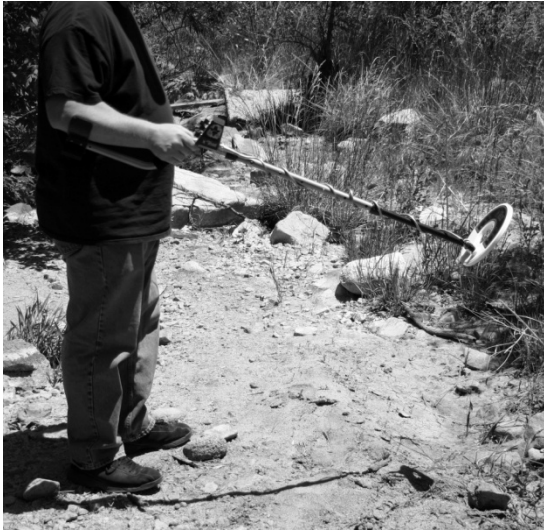
Figure 13 – Do Not Tilt the Searchcoil at an Angle to the Ground
