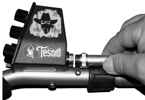
Figure 7 – Connecting the Cable
