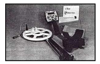
Assembling the Cortés is simple and requires no special tools. Just install the battery packs, mount the searchcoil on the lower pole assembly, connect the pole assemblies together, wrap the excess cable around the pole and plug the cable into the control housing. Finally, adjust the pole length and searchcoil angle and you're ready!
