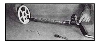
Your strongest signal will always be closest to the center of the coil. Additional information can also be learned by the signal strength and pitch. A smaller or deeper target will give a less noticeable change in the threshold than a larger or more shallow target will give. Take some time and try all of your targets at different depths to find out how your detector sounds.
