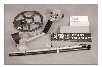
Assembling the Cibola is simple and requires no special tools. Just install the battery packs, mount the searchcoil on the lower pole assembly, connect the pole assemblies together, wrap the excess cable around the pole and plug the cable into the control housing. Finally, adjust the pole length and searchcoil angle and you're ready!
