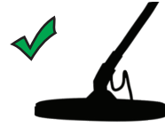
Correct search coil angle
