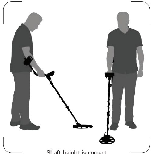
Shaft height is correct
