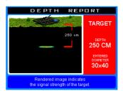
You can now begin by determining the dimensions of the target. To do this, move the coil towards the target. You will want to approach the target from the coil's side. Note that the front and rear parts of the coil are not used during measurement. Mark the first points at which you receive
