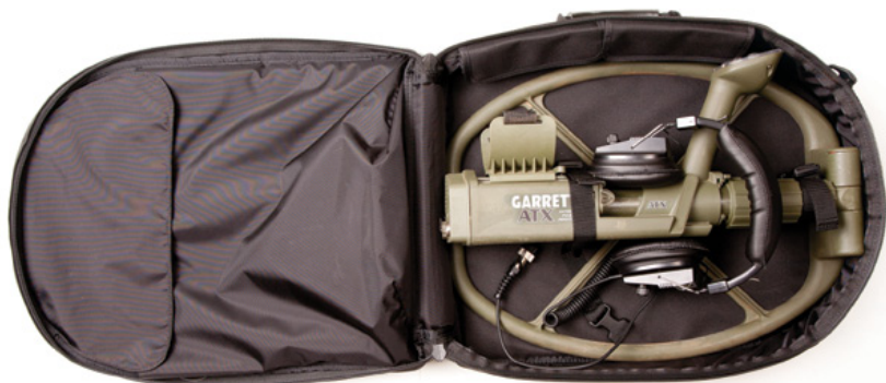
Figure 4: ATX with Deepseeker coil attached + headphones. Secure straps around lower stem nut and housing.
