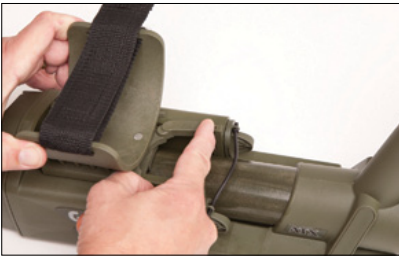
Armrest locking lever shown in open position.
