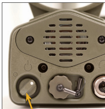
On/Off Switch (shown in On position)
