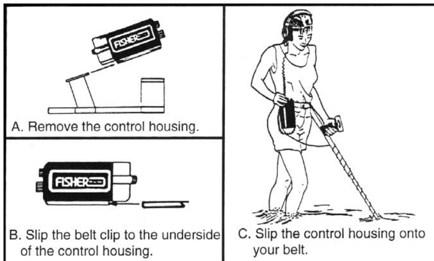
Figure 3. You can hipmount your 1280-X by sliding the control housing from the handle and attaching it to your belt. This reduces the weight of the stem, creating nearly effortless hunting.
