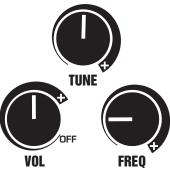
**HEADHUNTER PULSE** models have three controls for the operation of the special designed, highly sensitive, Pulse Induction circuitry. This circuitry is located in one of the sealed earcups of the headphones. Batteries are located in the other earcup, and are user accessible.
