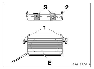
Unscrew both knurled-head bolts (1) and remove the holder (2) from the speaker **E**.
