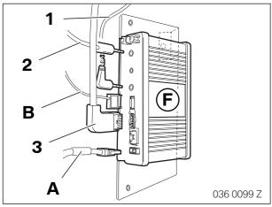
Connect the microphone cable plug (1), the speaker cable plug (2), the mobile phone holder plug (3) and branches **A** and **B** to the hands-free control module **F**.
