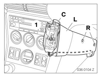
Do not damage the cable as you secure the telephone console. ◀
