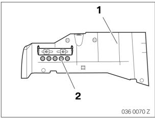
Drill the sound outlet holes (2) as shown in the bottom trim (1) with a 16 mm peel drill.
