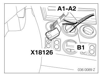
Lay branches A1 - A2 and B1 to the radio plug X18126.
