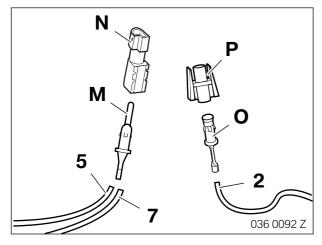
Cut the corresponding cable of the plug **X18126** at a suitable point.
