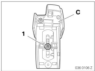
Remove the Philips screw (1) and take the mobile phone holder **C** off the retaining plate.
