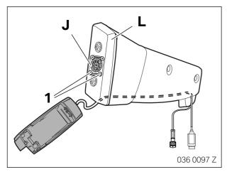
Place the retaining plate **J** on the top section of the telephone console **L** and mark the fixing holes.
