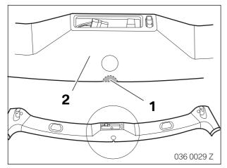
File out the cable passage hole (1) near the interior light with a round file in the windscreen panel trim (2).
