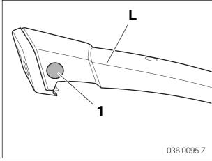
Drill the cable passage (1) for the mobile phone holder in the bottom section of the telephone console  $\mathbf{L}$  as shown using a 22 mm peel drill.
