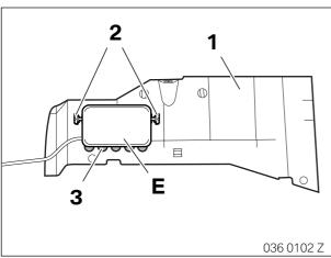
Insert the speaker **E** into the bottom trim (1) so that the speaker opening points towards the noise outlet opening (3). ◀
