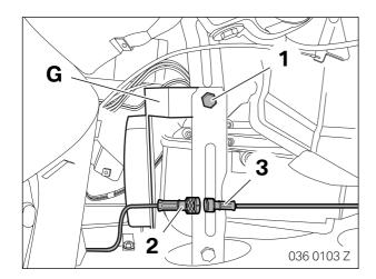
Secure the hands-free control module and holder **G** to the retaining screw (1).
