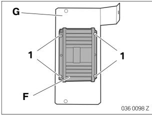
Place the hands-free control module **F** on the holder **G** and mark the fixing holes.
