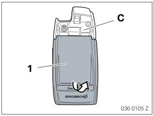
Remove the bottom section (1) from the mobile phone holder  ${\bf C}$ .
