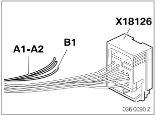
Connect branches **A1 – A2** as follows to the cables in plug **X18126**:
