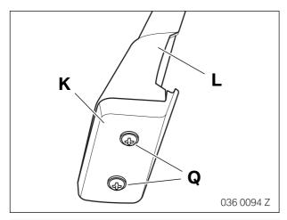
Connect the bottom section of the telephone console L to the top section K.
