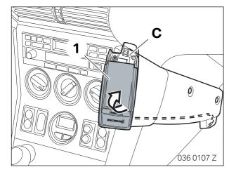
Position the bottom section (1) on the mobile phone holder  ${\bf C}$ .
